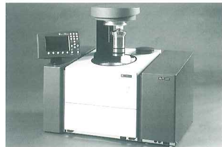
Ill. 2: IKA C 5000 with dry cooling system
